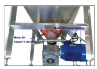
Two motors: one for screw feeding, one for hopper's vibrating
