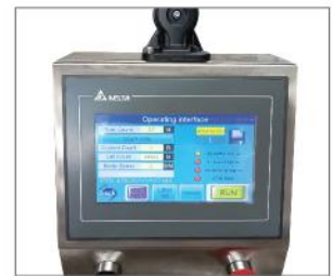
Local PLC and touch screen brand (Delta)
