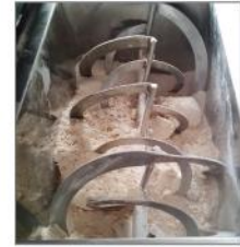
Powder contact fully with the blade to run the mixing as we as outlet.
