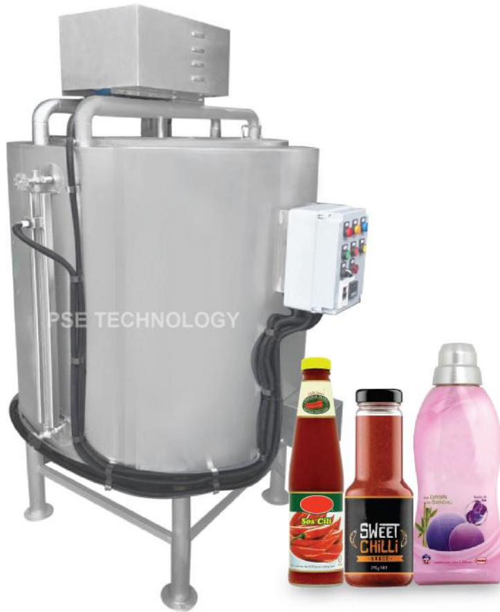
Local control panel box (Digital temperature controller)
