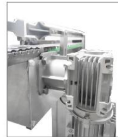
Strong motor fixing plate prevent conveyor crack down
