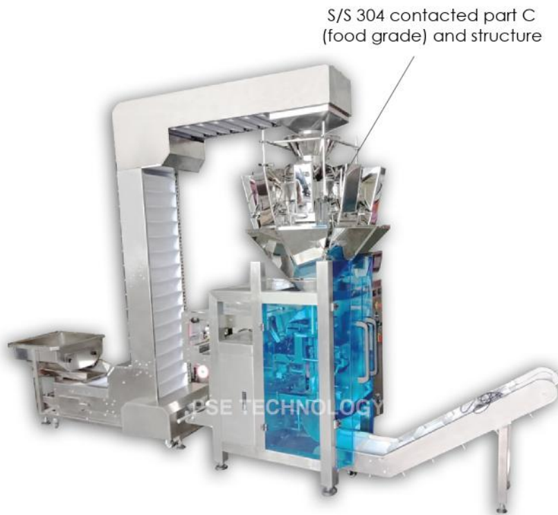
Optional: Product elevator to lighten the job pressure
