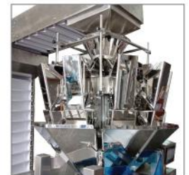
Precise granular filling by ten loadcell weigher
