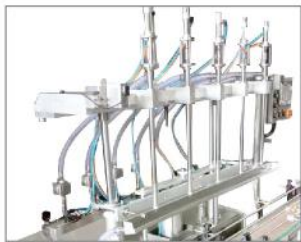
Nozzle filling with stopper design to improve accuracy and prevent dripping
