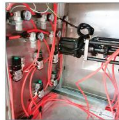
New cylinder air mechanical mechanism - More easy to adjust and service than old CAM type
