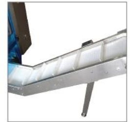
Optional: Output conveyor to collect product to packing area
