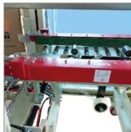
Easy adjustment for different carton size
