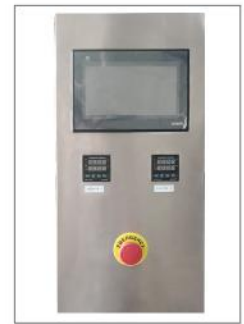
OMron touch screen control + PLC (local standard)
