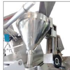
- Precise auger system - S/S 304 material
