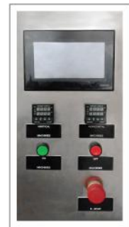
Omron touch screen control + PLC (local standard)
