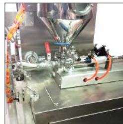
- Precise auger system - S/S 304 material
