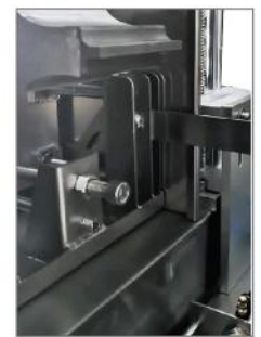
Solid holder to ensure good sealing effect
