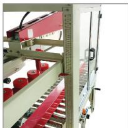
Door to ensure safety work environment
