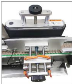
Easy adjustment design for different bottle shape
