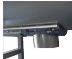
Simple outlet bottom to avoid powder residue with old design.
