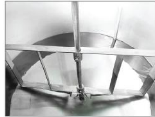
Agitator mixing blade U shape to create uniform mixing
